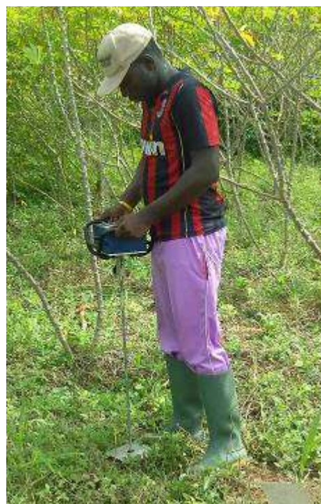
Figure 3. The Eijkelkamp penetrometer in operation.
