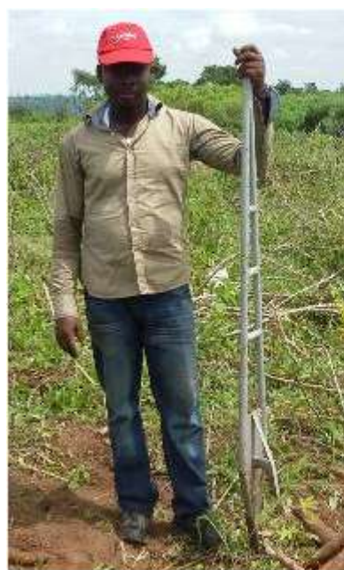
Figure 2. The improved manual cassava harvesting tool.
